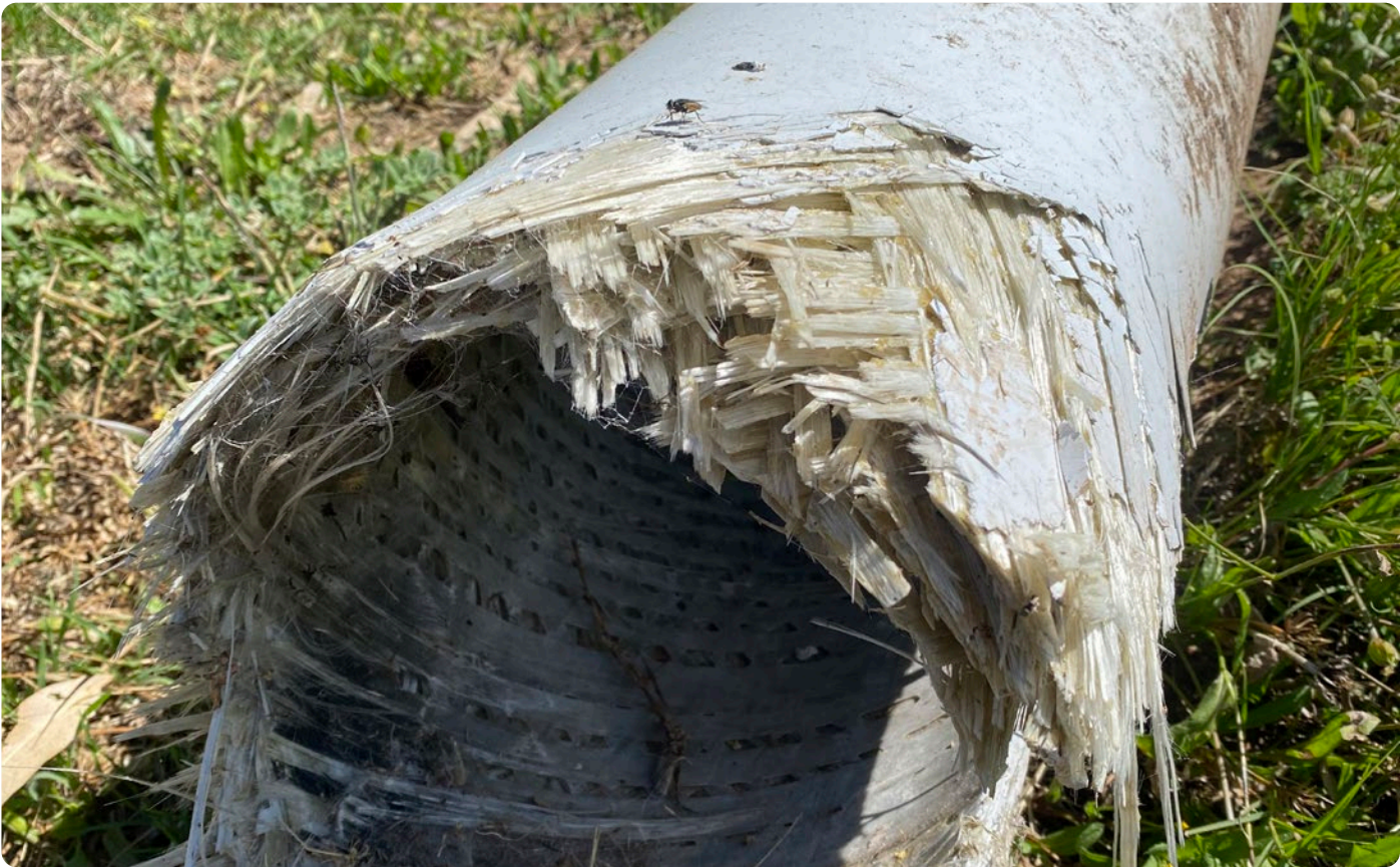
Figure 2.11: Street poles are made using filament winding.
