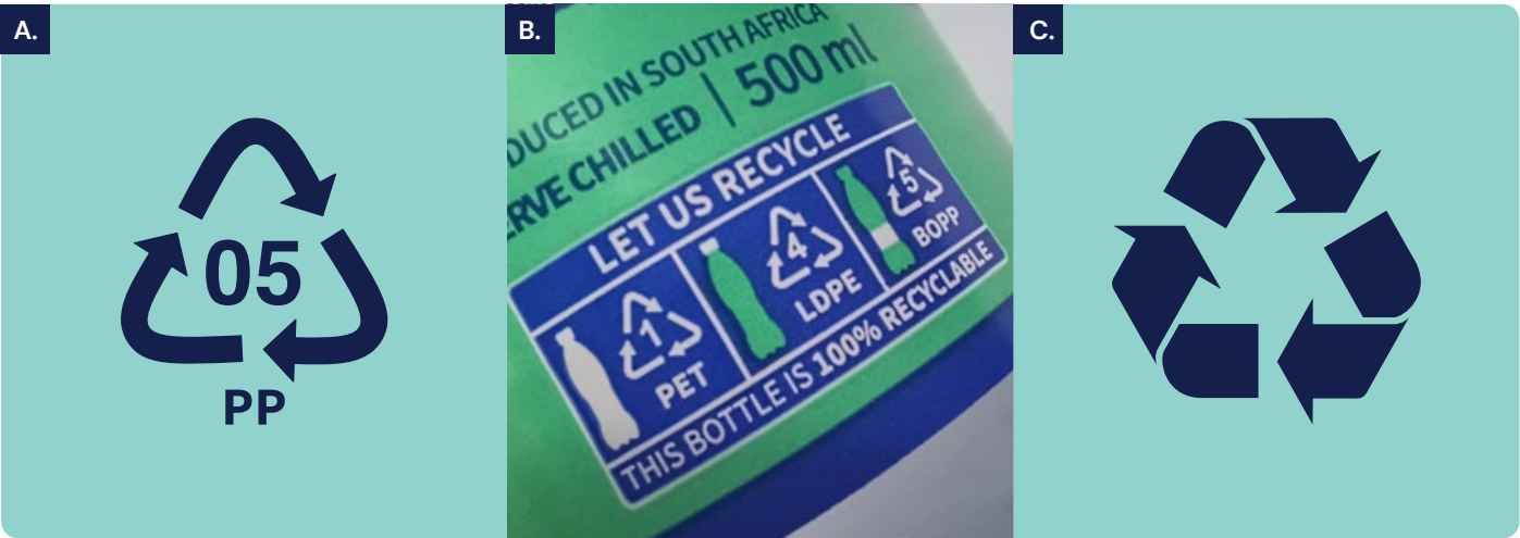
Figure 1.3: Example of material identification codes. A) The code for PP, one of the commodity plastics. B) Sometimes, a producer will indicate the identification codes for each part of the packaging (a water bottle in this case), i.e., the bottle, the lid, and the label. “BOPP” indicates PP with biaxial orientation (see Section 1.4). C) The Mobius loop.
